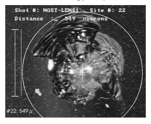
For this test the particle velocity was 5.6 km/s and its diameter, 57  $\mu$ . The crater and spall were nonsymmetric. The crater and spall dimensions were:  $Y_C = 103 \ \mu$ ,  $D_C = 63x90 \ \mu$ ,  $Y_S = 51 \ \mu$ , and  $D_S = 740x780 \ \mu$ .
